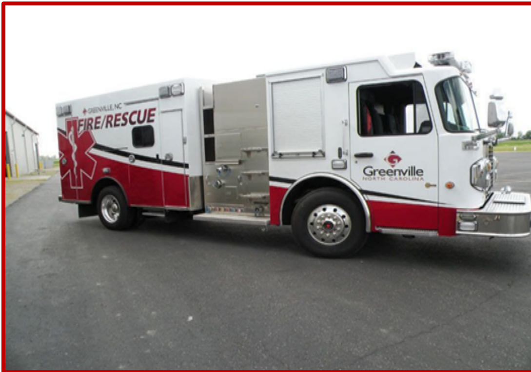
Figure VI-7: Multipurpose Combination Fire Suppression/EMS Transport Vehicle
